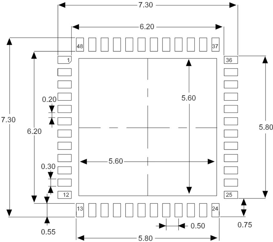
Note: Dimensions are marked in millimeters.
