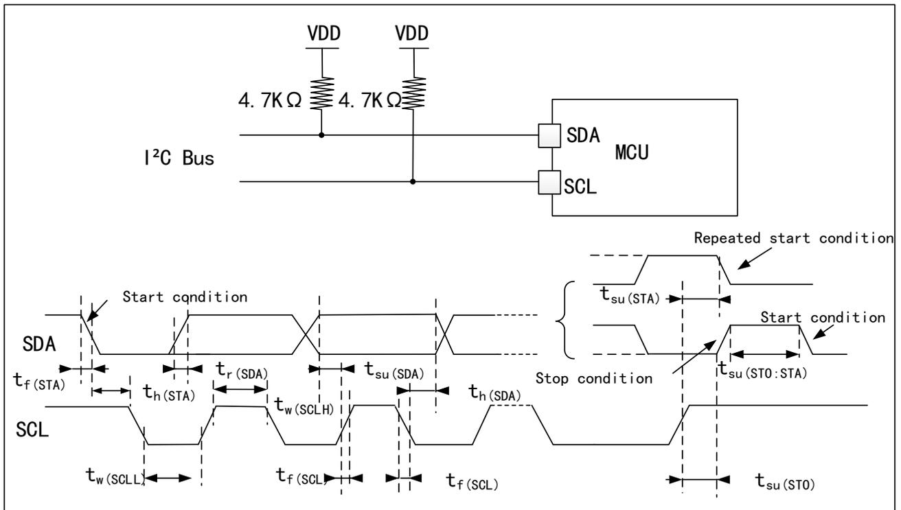
Note: the measuring points are set at CMOS levels: 0.3V<sub>DD</sub> and 0.7V<sub>DD</sub>.
