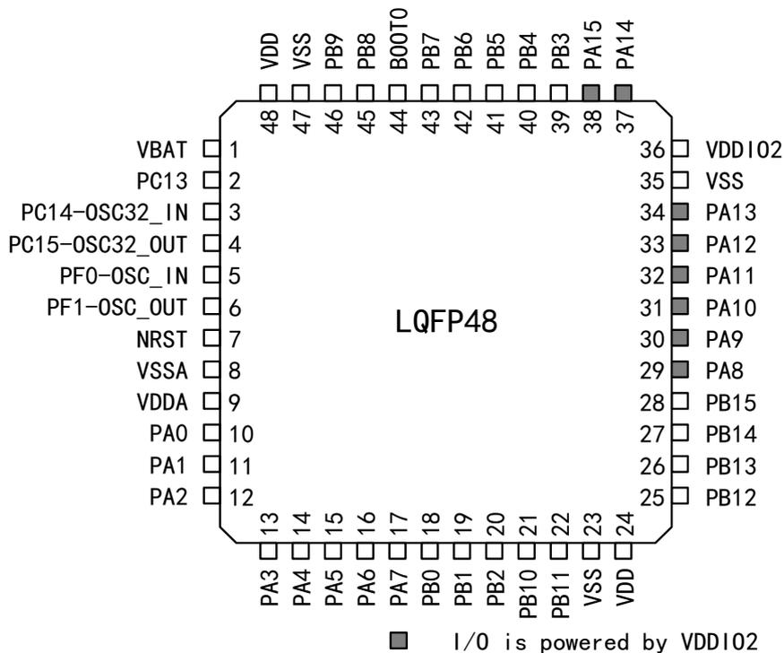
Figure. 4 Pin Distribution Diagram of APM32F072x8xB Series QFN48
