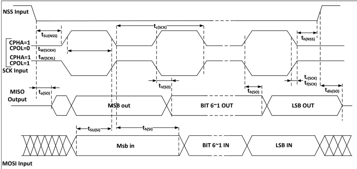
Note: the measuring points are set at CMOS levels: 0.3V<sub>DD</sub> and 0.7V<sub>DD</sub>.
