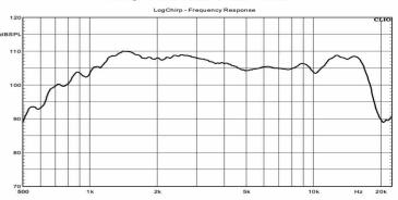
Test conditions: 1W/1m standard test box in anechoic chamber.
