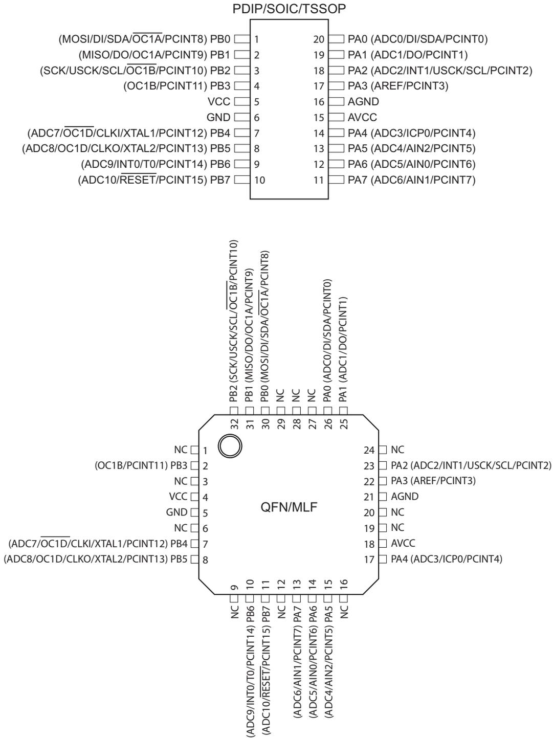
Note: To ensure mechanical stability the center pad underneath the QFN/MLF package should be soldered to ground on the board.
