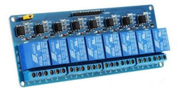
The default delivery 5 v relay relay. 8 road relay module
