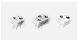
Block-type BNP002 filters completely eliminate noise from extremely wide frequency bands. The BNP002 is ideal for eliminating noise in logic signal circuits and is designed to perform superbly through the use of through-type barrier layer capacitors, and bead inductors.
