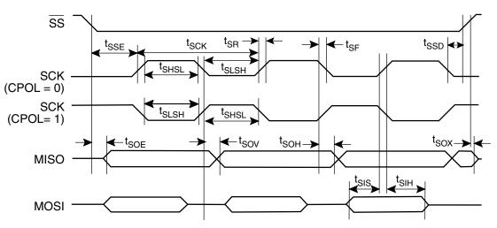
Figure 15-6. SPI Master Timing (CPHA = 1)
