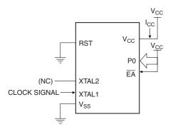
43. I<sub>CC</sub> Test Condition, Idle Mode, All Other Pins are Disconnected
