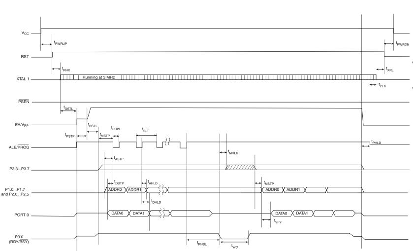
Figure 27-1. Flash/EEPROM Programming and Verification Waveforms – Parallel Mode
