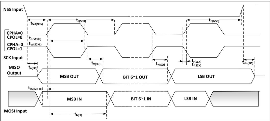
**Figure 15 SPI Timing Diagram - Slave Mode and CPHA=1**
