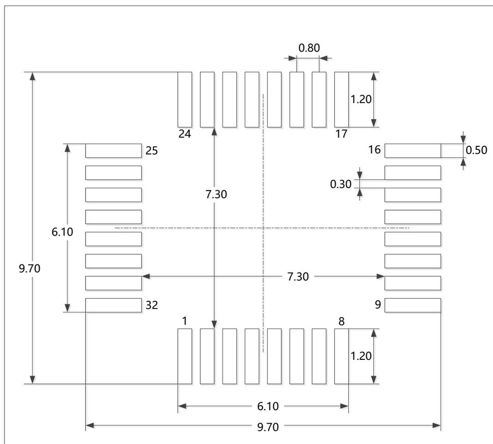
**Note:** Dimensions are marked in millimeters.
