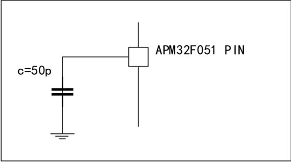
**Figure 10 Pin Input Voltage Measurement Scheme**
