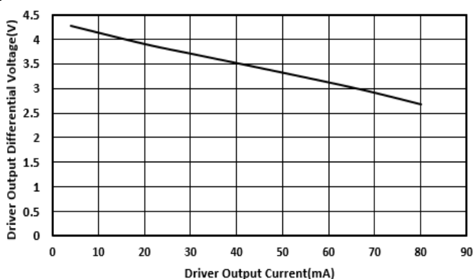
Figure 7-2 Driver Differential Output Voltage vs Driver Output Current
