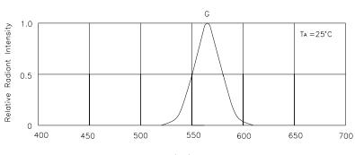
$\label{eq:wavelength} \begin{tabular}{ll} wavelength & $\lambda$ (nm) \\ \hline {\it RELATIVE INTENSITY Vs. WAVELENGTH} \end{tabular}$
