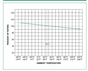
1. Re-rating depicted in this curve is in addition to the standard re-rating of 25% for continuous operation.
