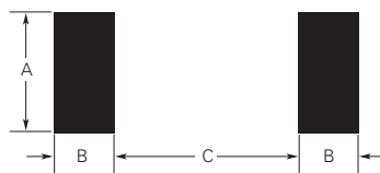
Figure S14 Recommended Pad Layout for Surface-mount Devices
