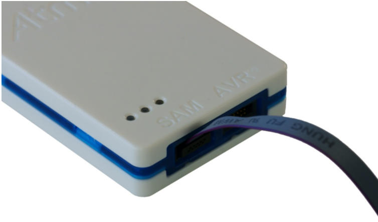
Figure 2-11. Atmel-ICE SAM Probe Connection
