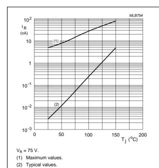
Fig.5 Reverse current as a function of junction temperature; per diode.
