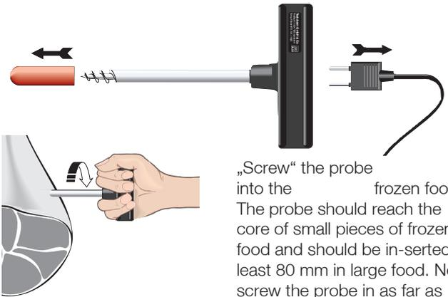
„Screw“ the probe into the frozen food. The probe should reach the core of small pieces of frozen food and should be inserted at least 80 mm in large food. Never screw the probe in as far as the handle.
