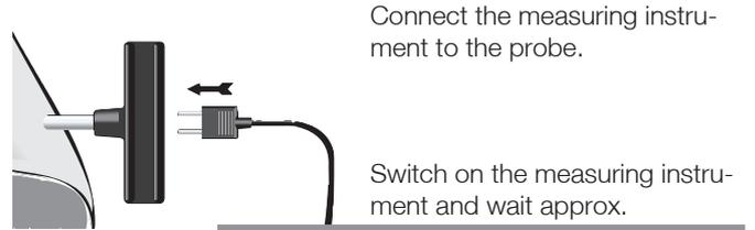
Connect the measuring instrument to the probe.
