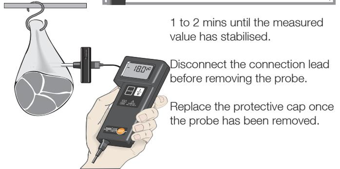
1 to 2 mins until the measured value has stabilised.
